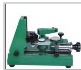
inspect accuracy of test indicators
