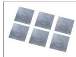
A1 standard sensitivity test piece (optional)
