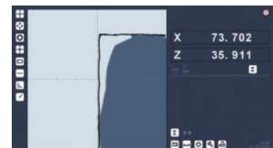
scanning the maximum profile of cutting tools
