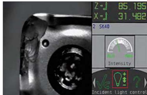
check cutting edge wear
