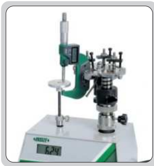
check the measuring force of micrometers
