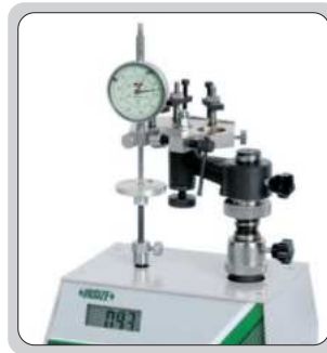
check the measuring force of dial indicators
