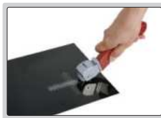
step 1: make grid cutting on surface
