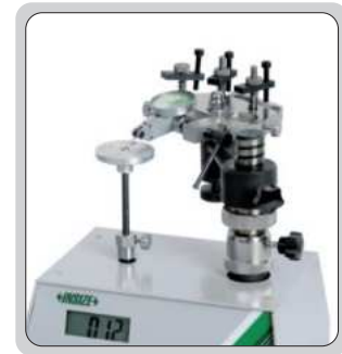
check the measuring force of dial test indicators
