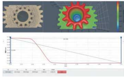
measurement of component bore height
