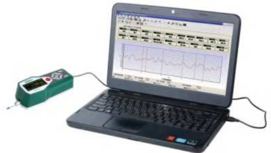
operate roughness tester by computers
