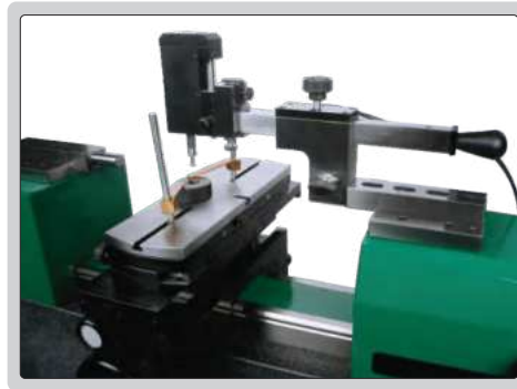
thread ring gauge measurement
