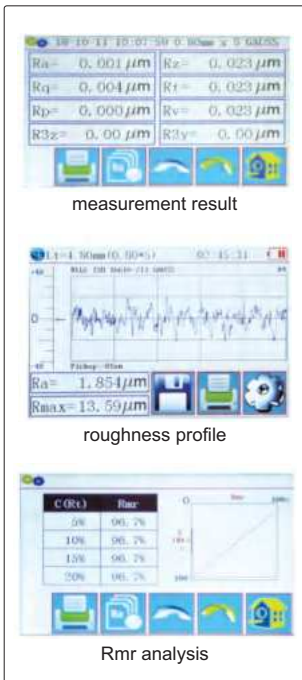
roughness tester screen display
