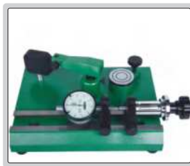
inspect accuracy of dial indicators (range 0-25mm)
