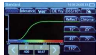
specimen reflectance recording interface
